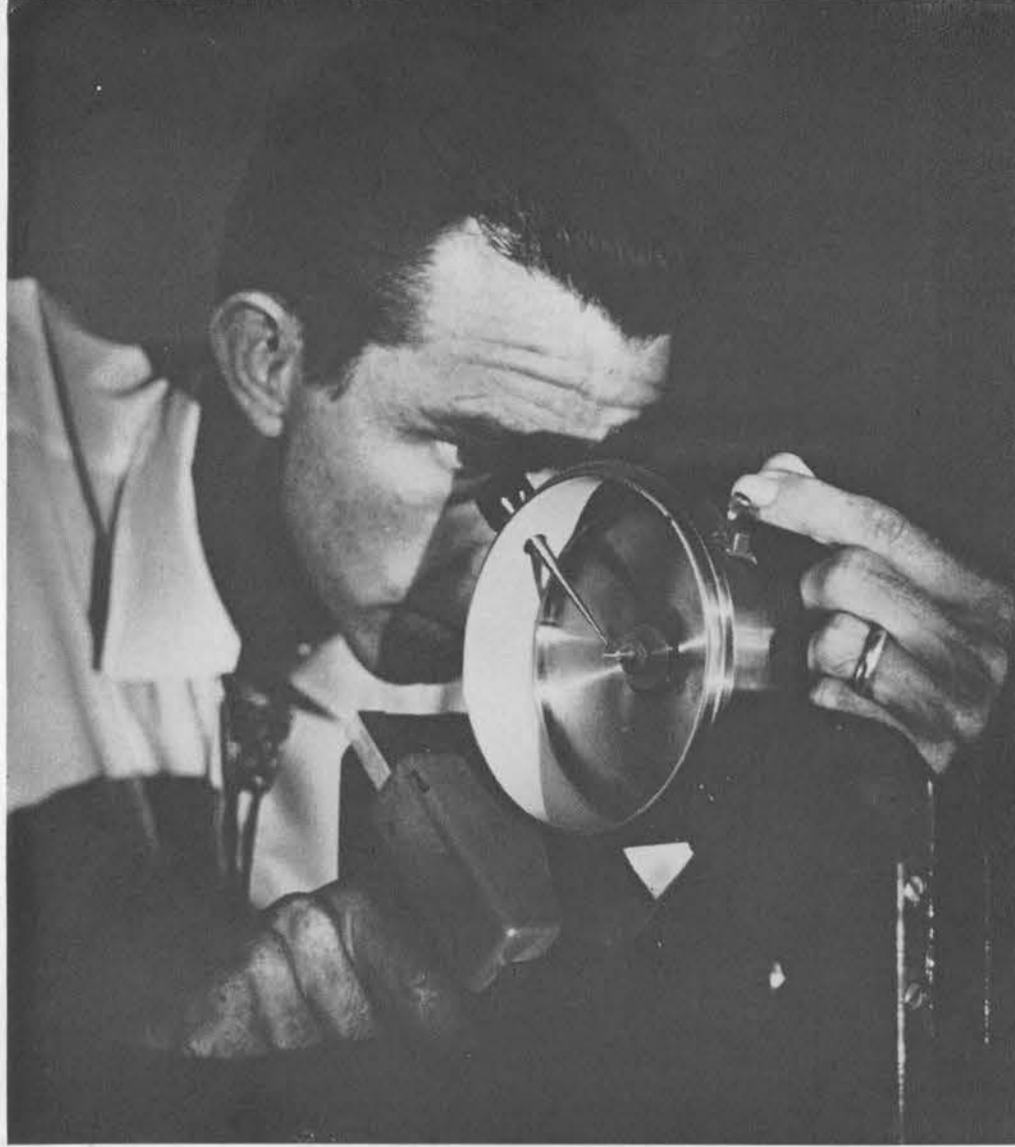
PRECISE ALIGNMENT of sample material in a Debye-Scherrer camera is necessary to make accurate diffraction patterns. J. R. Woodworth (1122) makes adjustments to insure that X-ray beam will strike sample material mounted at center of Debye-Scherrer camera.
